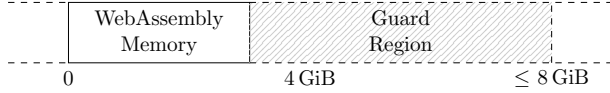
Figure 1. Memory layout for 3 GiB of accessible Wasm memory. The hatched region represents inaccessible memory, protected from illegal accesses using guard pages.
